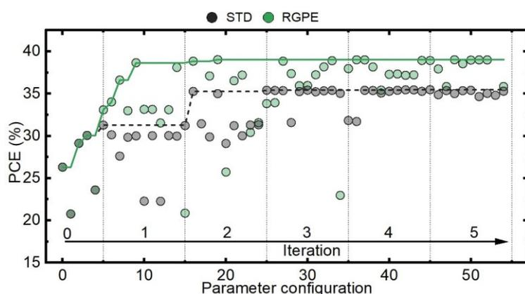
Figure: Exemplary optimization progress of tandem solar cell's PCE using BO methods in this work. Circles represent obtained PCE within a batch. Lines show the maximum obtained PCE.
