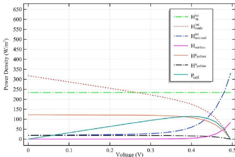
Fig. 1, The power density of all heat generation factors versus voltage
