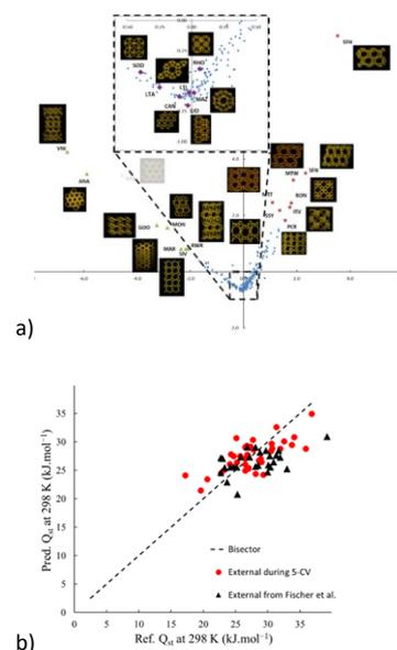
Fig. 1.a V-Shape classification map of the International Zeolite Assoc. (IZA) database. b) Parity plot of isosteric heat of adsorption of CO<sub>2</sub> on IZA zeolites predicted using Support Vector Machine (SVM) and our descriptors
